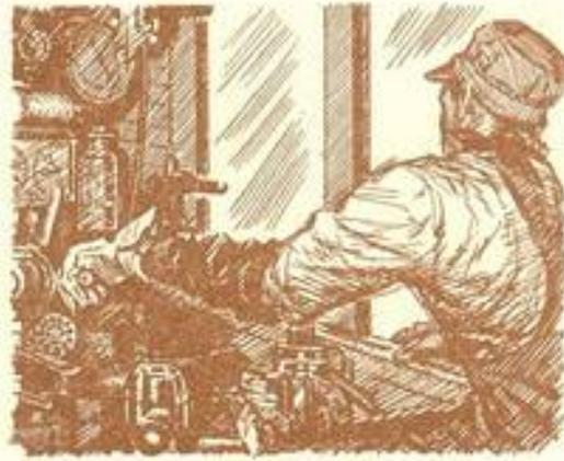
**Now the *Daylight* engine gently couples onto the train at the station, the air hoses are connected and a terminal brake test is made. The engineer charges the air line to the required pressure and applies the brakes. Car inspectors then check the train, and make sure that all brake shoes clamp firmly against the wheels.**
